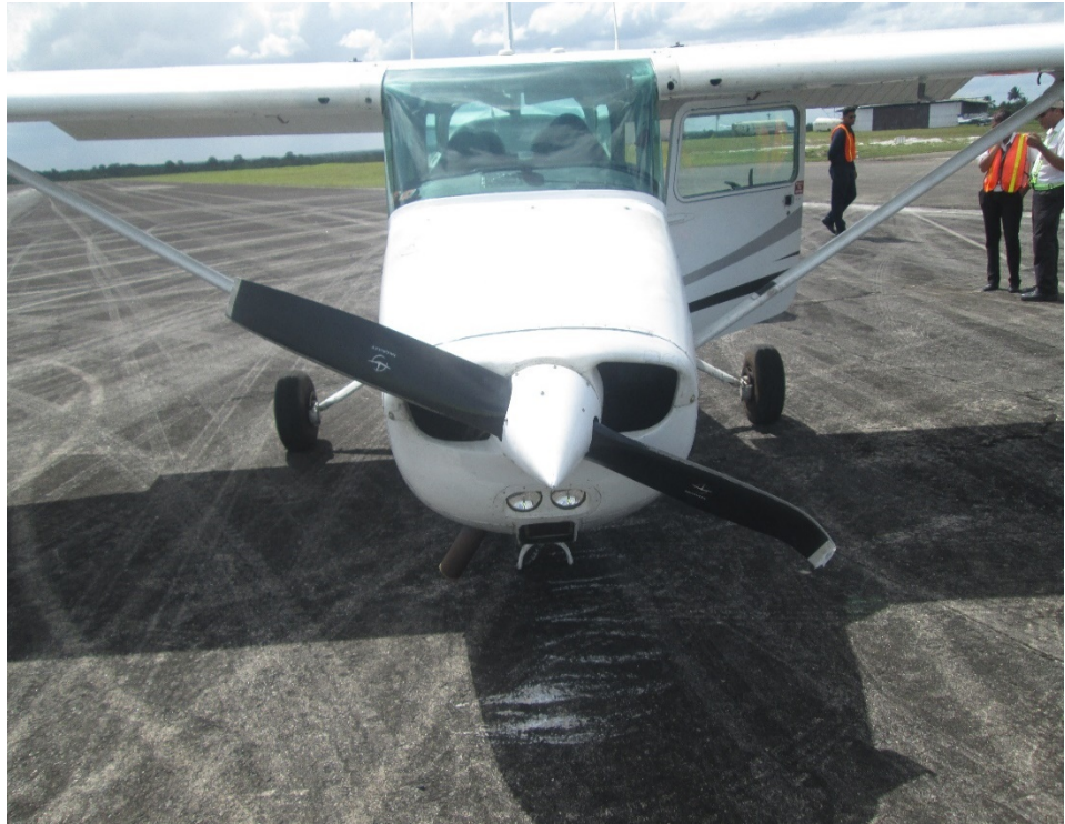
Picture #1 – showing damage to nose wheel fork and propeller blades
