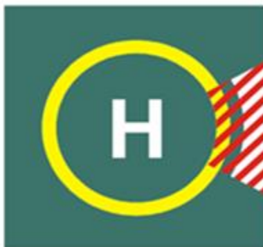
FIGURE 6-7: HELIDECK PROHIBITED LANDING SECTOR MARKING
